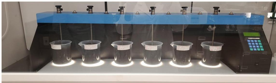
**Figure B-5.** Pictorial view of Jar test experiment for solid separation.
