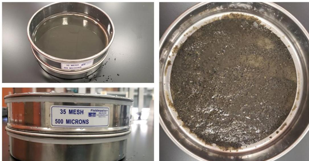
**Figure B-4.** Pictorial view of solid separation by sieving.
