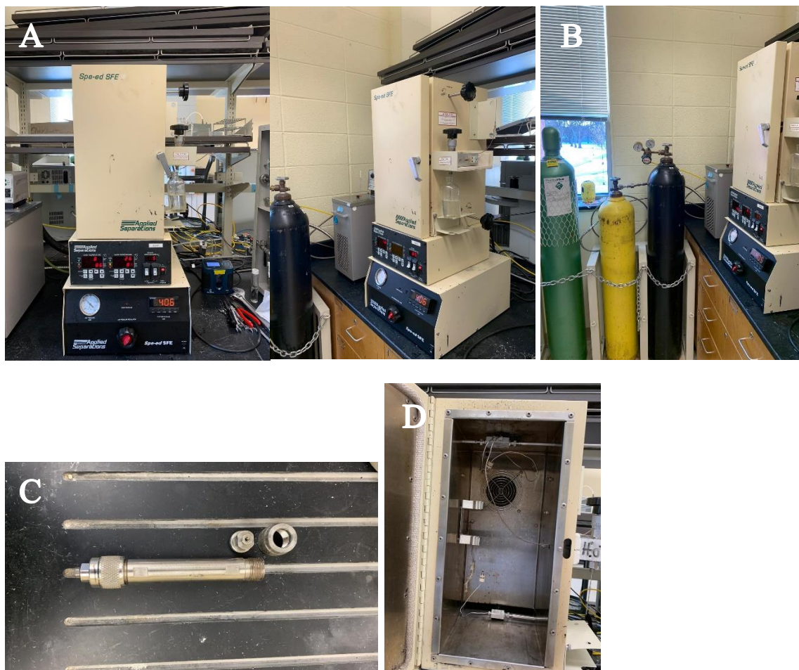
Figure 4. Supercritical fluid extractor (Spe-ed SFE, Applied Separation) (A) used in startch extraction. The system includes CO 2 cylinder (B), a 25 ml stainless steel vessel (C) and an oven (D).
