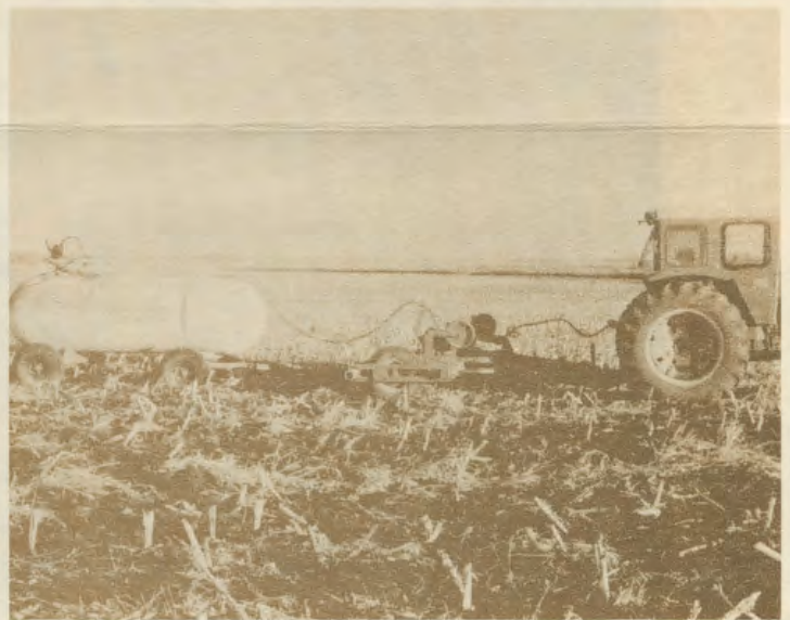
Anhydrous ammonia application and chisel plow tillage can be combined into one operation.
