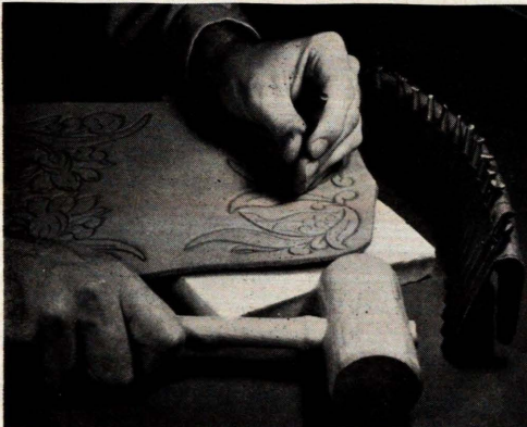
Beveling the carved design—note position of tool.
