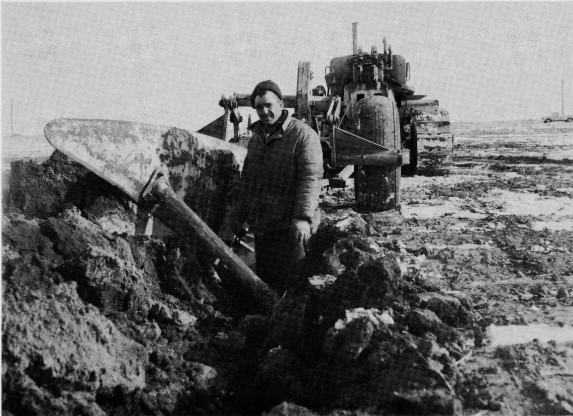
This plow can break to 30 inches; Aberdeen claypan is between 9 and 21. The plow required a crawler 8 years ago; modern tractors could handle it.
