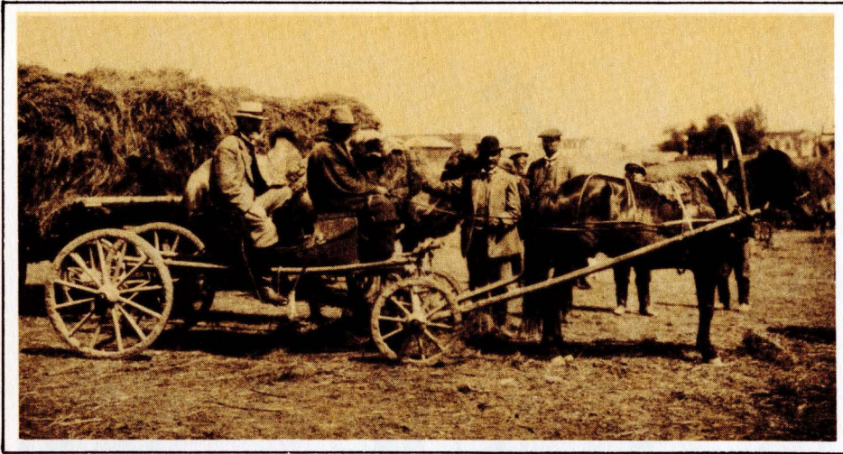
Wooden wheels, no springs, the bed swung from wooden poles—this is the tarantass, the vehicle Hansen traveled in on some tours. Here the
