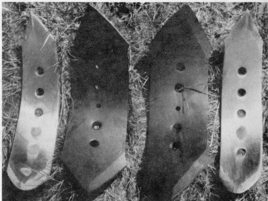
Pasture interseeding is a tested method for improving native range and tame pastures and haylands. Photos are explained clockwise from bottom right. South Dakota State University (SDSU) has developed this improved pasture interseeder shown at bottom right. Chisel plow shovels, shown bottom left, can be 4 or 6 inches wide. The wider shovel is used in dry areas or in heavy sod. SDSU's pasture interseeder is shown in use at top left. Next is a photo of the furrows made with the 6-inch shovel. In a closer view, these furrows are 8-9 inches wide and 3-5 inches deep. A 12-inch ruler is being held across the furrow. The furrow made by a 4-inch shovel is shown in the next photo. It is 5-6½ inches wide and 3-5 inches deep. Again, a 12-inch ruler is held across the furrow for comparison. An established interseeded native range is shown at top right.
