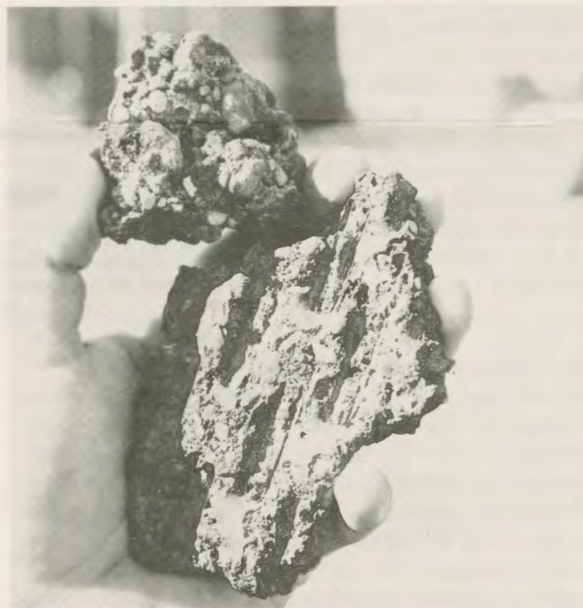
Figure 2. These incrustations were caused by precipitation of material carried up to the screen in solution.
