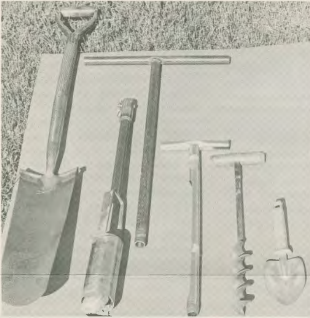
Several different tools (including some hydraulic equipment) can be used for taking deeper 6-24 inch as well as 0-6 inch samples.
