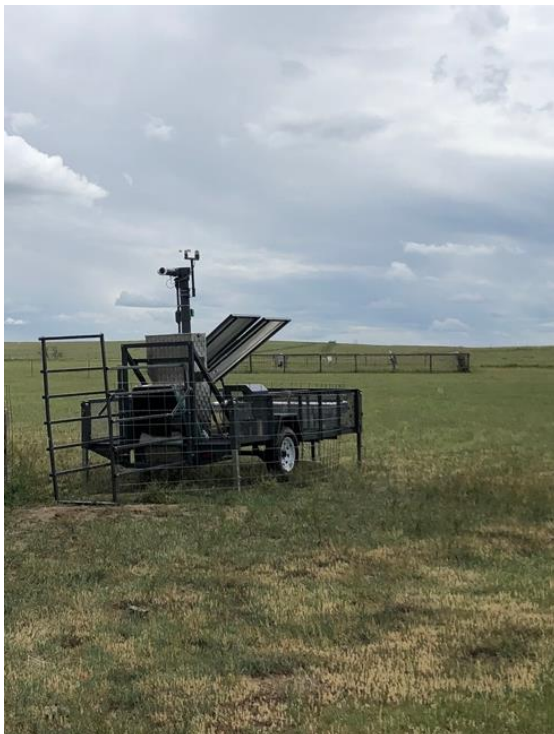
Fig. 3.1. Photo of GreenFeed™ pasture system 297 deployed in pasture. This system is placed on a trailer and is solar powered.
