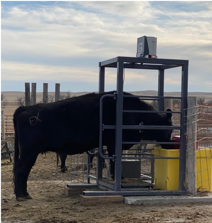
Fig. 3.5. Example of a cow using the SmartScale™ attached to the Ritchie Livestock Waterer in the drylot at the South Dakota State University Cottonwood Field Station (Cottonwood, SD).
