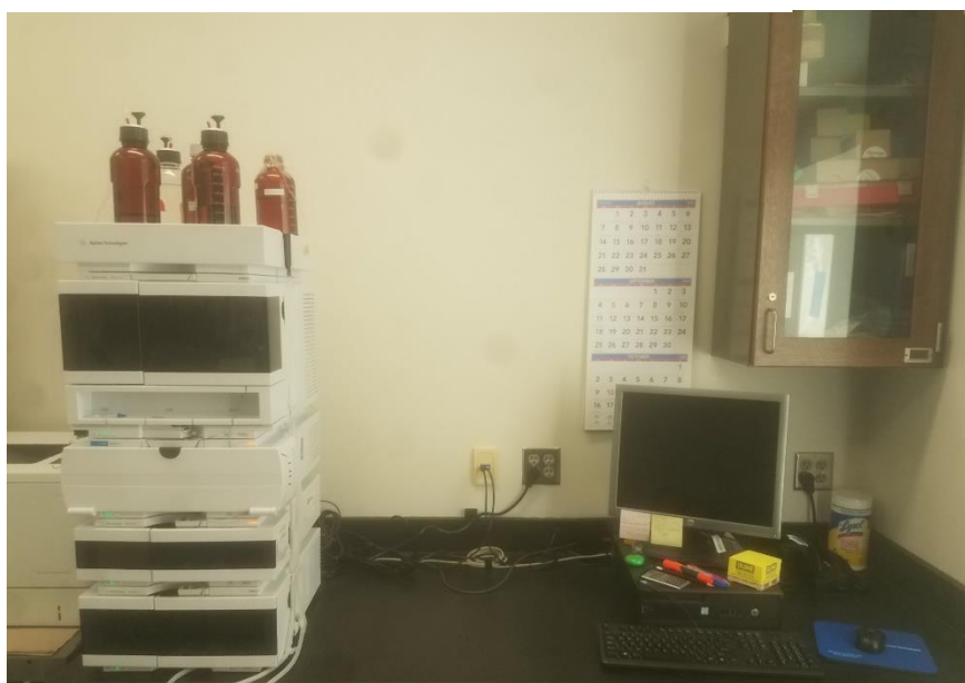
Figure 3. The complete set up of the HPLC machine at the South Dakota State Seed Testing Laboratory and the computer used to analyze results.
