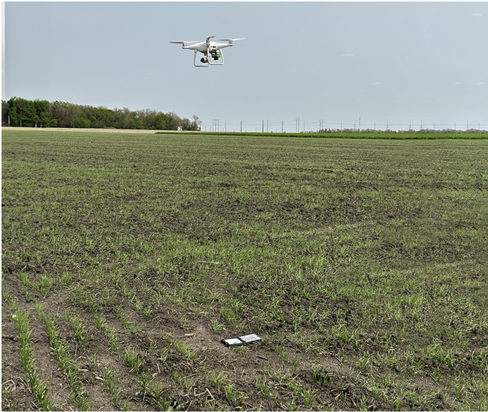
Figure 3.7: A drone, equipped with a multispectral camera, captures imagery over a calibration panel, ensuring precision in data on the image acquisition day.
