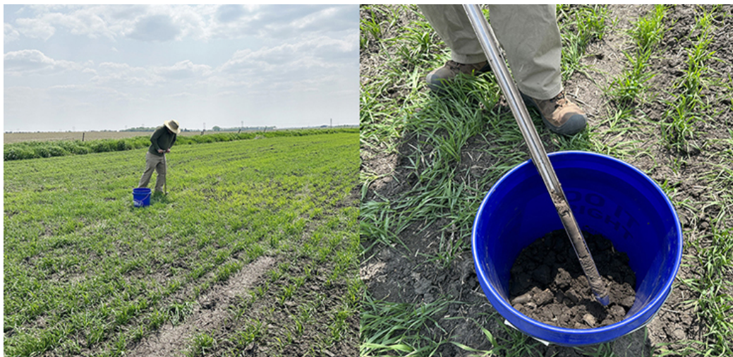
Figure 3.3: Soil Sampling Process. On the left, a researcher is shown in the field, actively using the auger for soil sampling. On the right, a soil auger is depicted with a freshly extracted soil sample.
