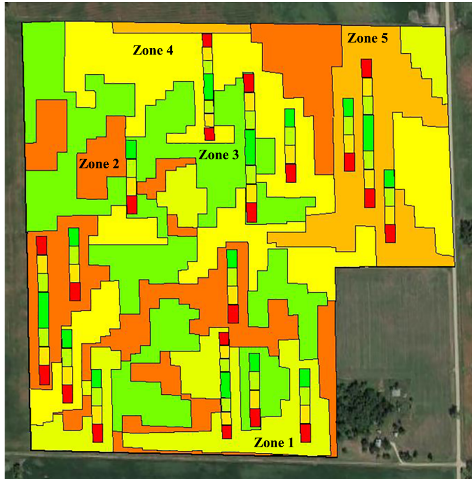
Figure 4.16: Layout of the nitrogen application test strips in the Mount Vernon field. Each strip is segmented into four plots, with each plot receiving a unique nitrogen application rate to assess the impact on crop performance. The strips are replicated across each zone to ensure representation of the field's variability.
