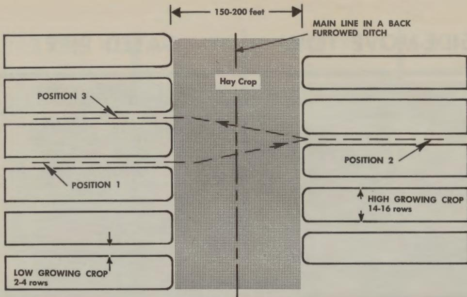
Figure 1. Field layout for tow-line sprinkler system.
