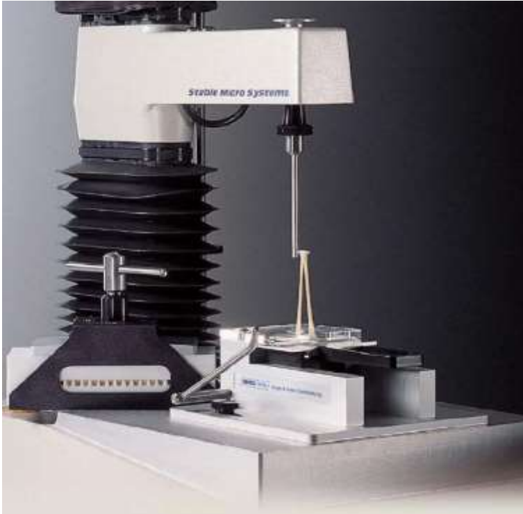
Figure 12. SMS Kieffer Dough and gluten extensibility rig.
