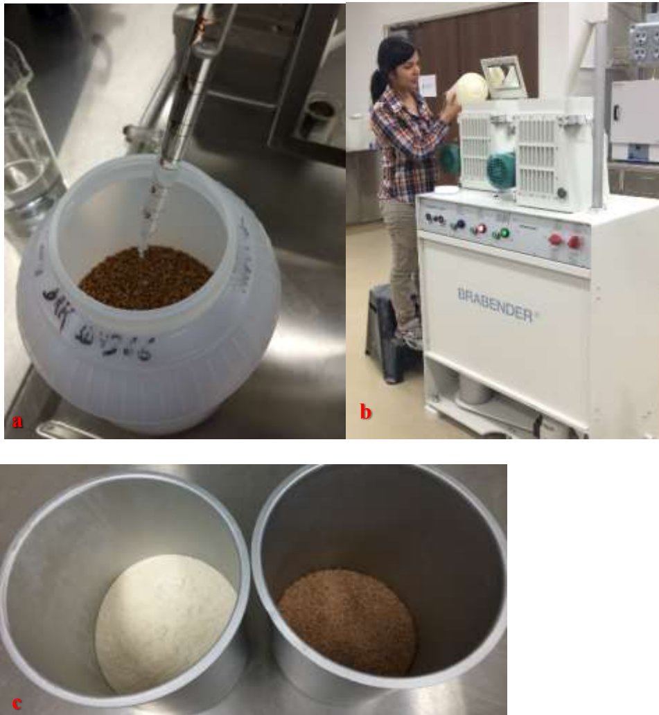
Figure 10. (a) Tempering of whole wheat (b) wheat milling (c) white flour (left) and wheat bran (right) obtained after milling.
