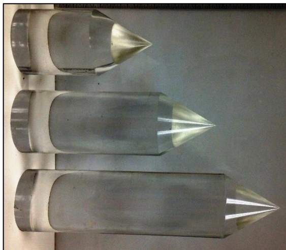
Figure 3.9. Light guides with different lengths (101.6 mm, 152.4 mm and 203.2 mm)
