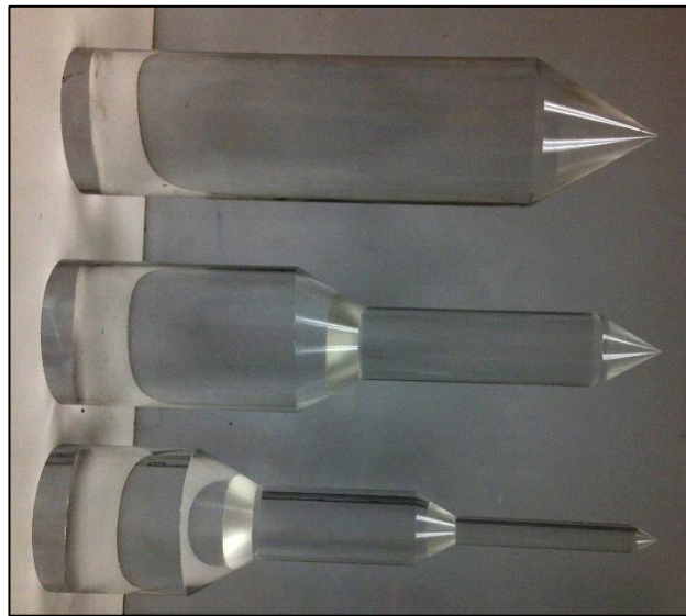
Figure 3.8. Simple and compound light guides
