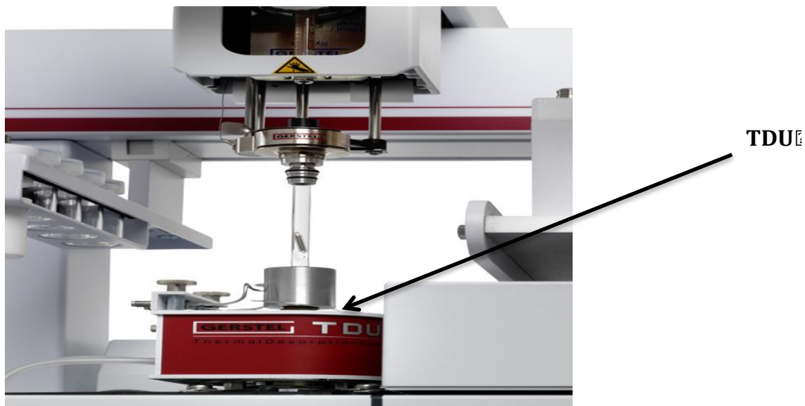
Figure 1.5. Thermal Desorption Unit (TDU) [37].
