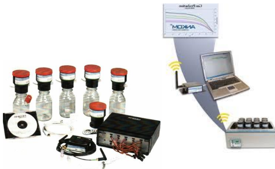
Figure 2.1. Components of Ankom in vitro Gas production measurement system (ANKOM Technology, 2012)
