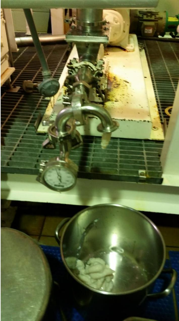
Fig 3.2 Positive displacement discharge pump during experiment.
