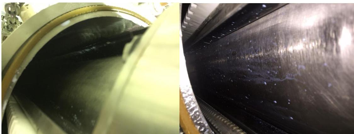
Figure 3.4 Rotor assembly post evaporation prior to full cleaning, but after water rinse.
