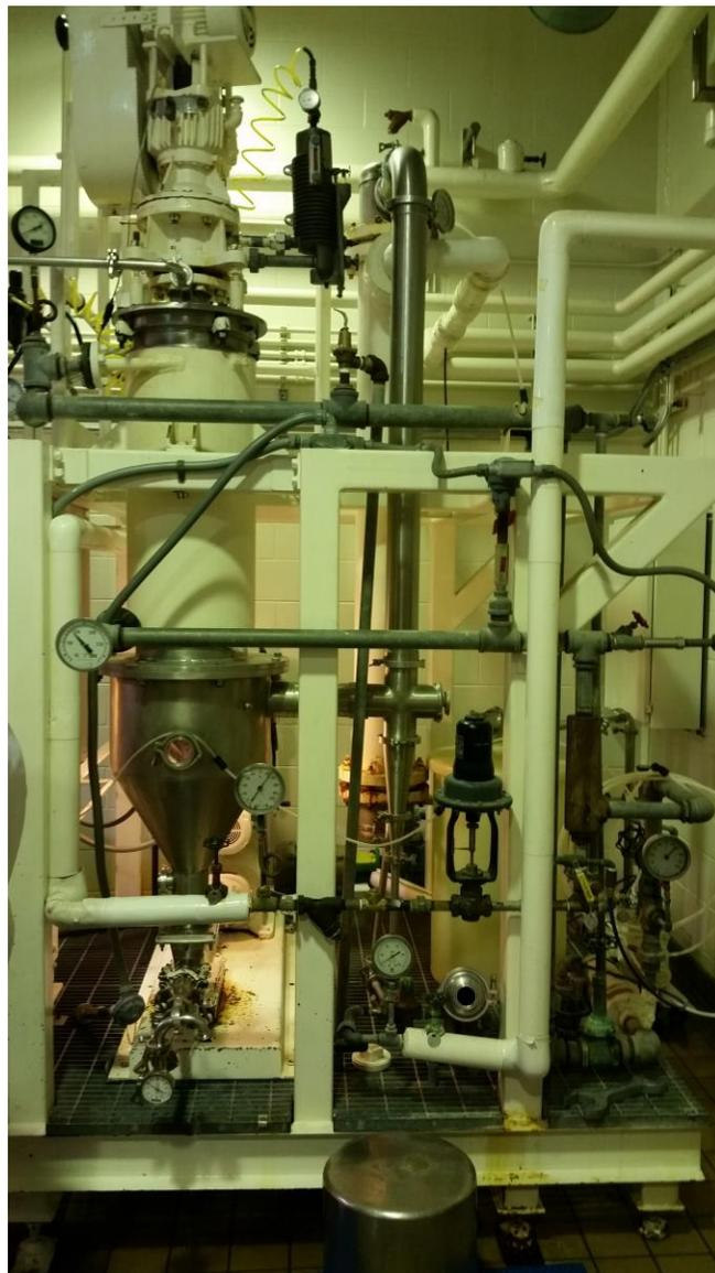
Fig 3.1 Pfaudler WFE used in the evaporation of MCC
