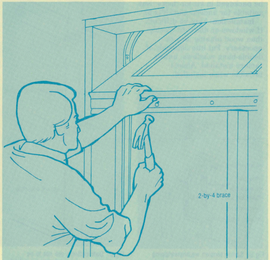
Fig 14. Garage door weatherstripping is easy to install. Put the thicker edge to the outside. Metal and fiberglass doors come with weatherstripping factory installed, but
