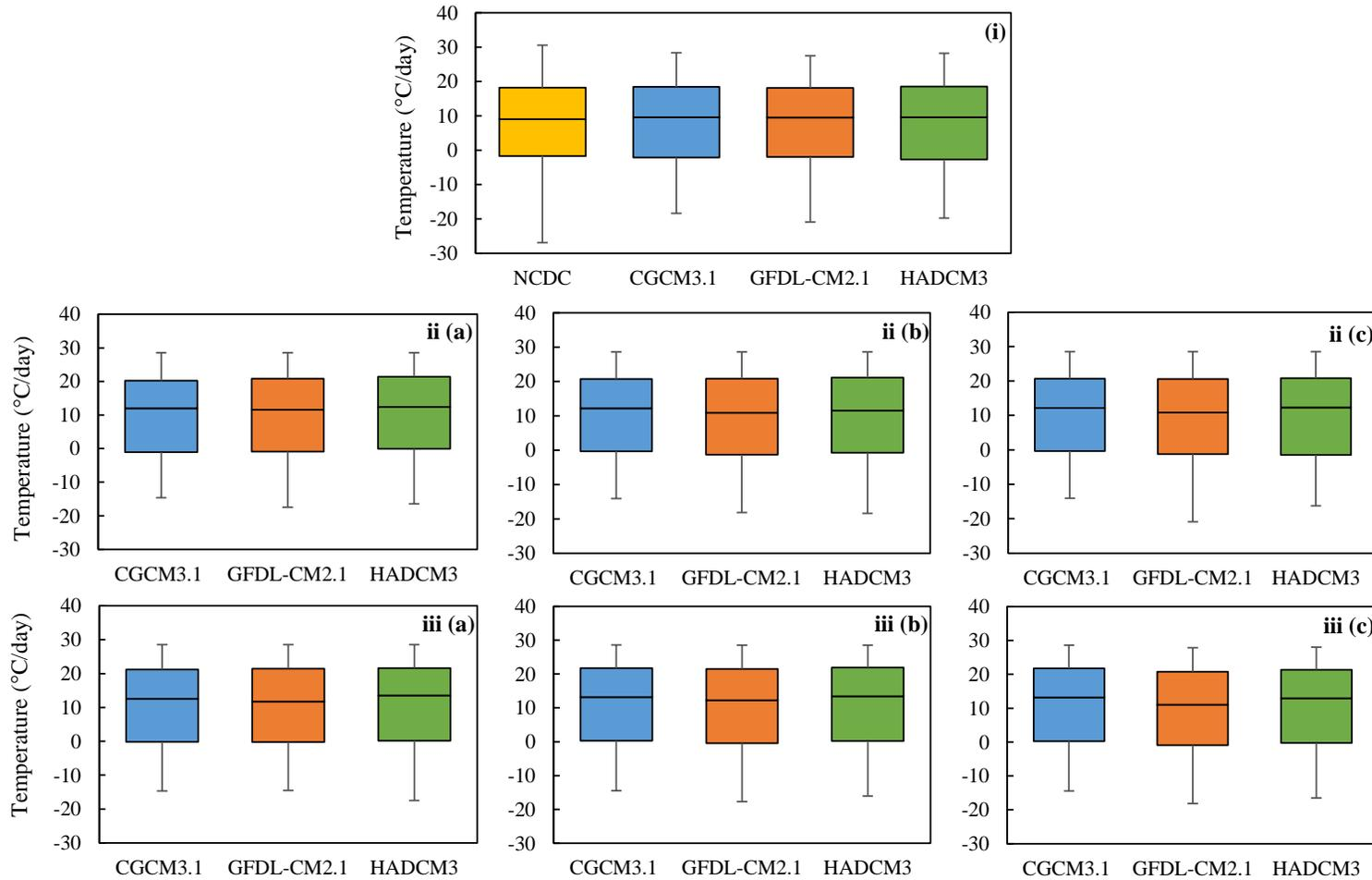
Figure 4. 6a: Projected maximum temperature for 1) baseline (1981-2000), 2) mid-century (2046-2065) and 3) end century (2080-2099) under the a) A1B, b) A2 and c) B1 scenarios.
