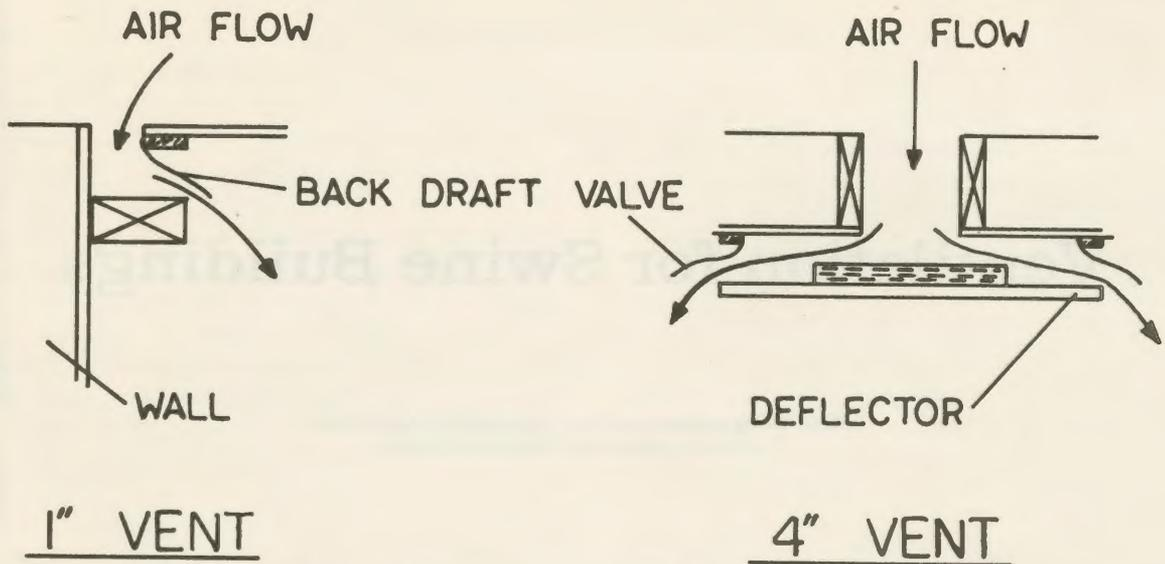
Figure 2. Slot intake construction in buildings up to 32 feet wide (left). Slot intake construction in buildings more than 32 feet wide (right).
