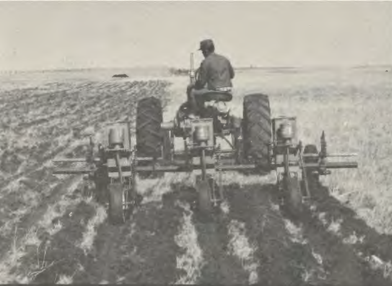
Seeding practices may be drilled or interseeded with special equipment under the Program.
