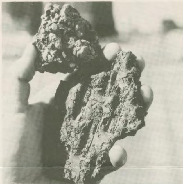
Figure 1. These incrustations were caused by precipitation of material carried up to the screen in solution.
