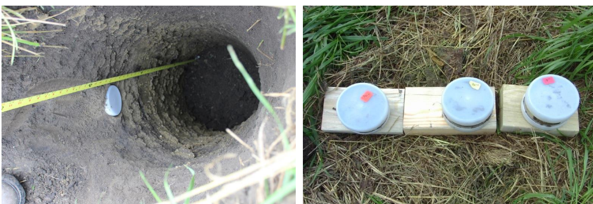
Figure 13. Soil sampling rings for undisturbed soil sample collection.
