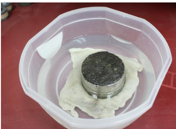
Figure 14. Soil sample saturation process.
