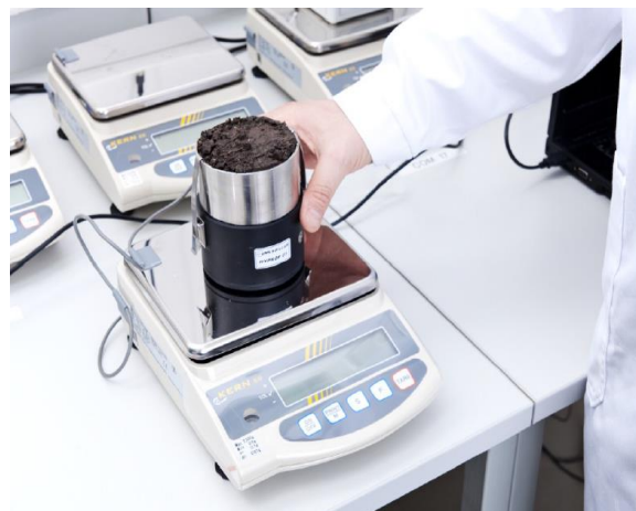
Figure 17. HYPROP base with tensiometer ready for reading.
