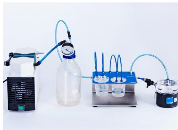
Figure 15. De-airing of HYPROP and tensiometer.
