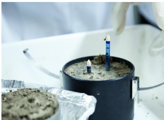
Figure 16. Tensiometer fitted with HYPROP base.
