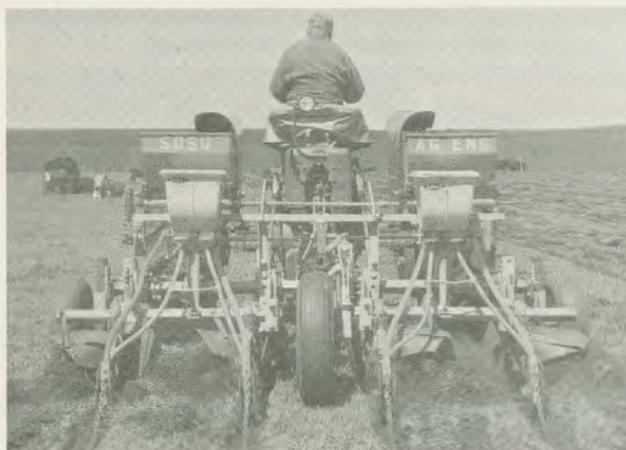
Fig. 3. Interseeder in operation on bluegrass pasture in Lincoln County. Note two sets of seed boxes.
