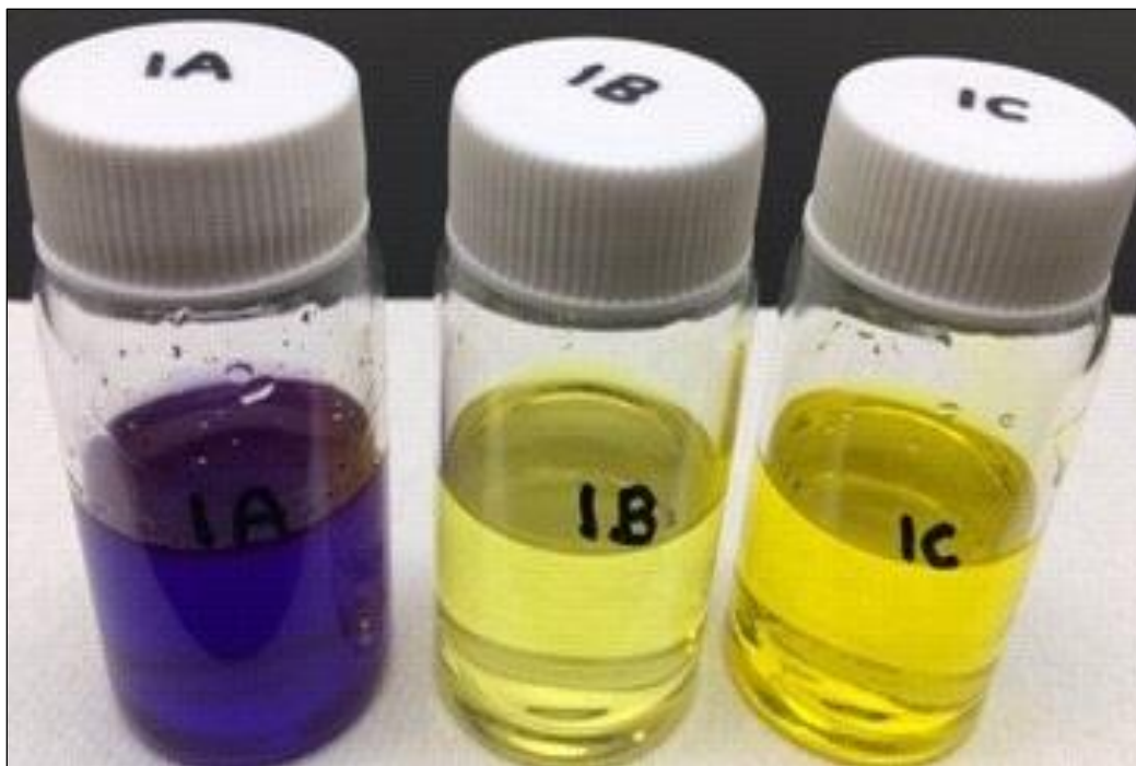
Figure 4.3. Violet, light yellow and yellow colors of Nile Red, 4-nitroaniline, and N, N-diethyl-4-nitroaniline dyes respectively (left to right) dissolved in DES01.
