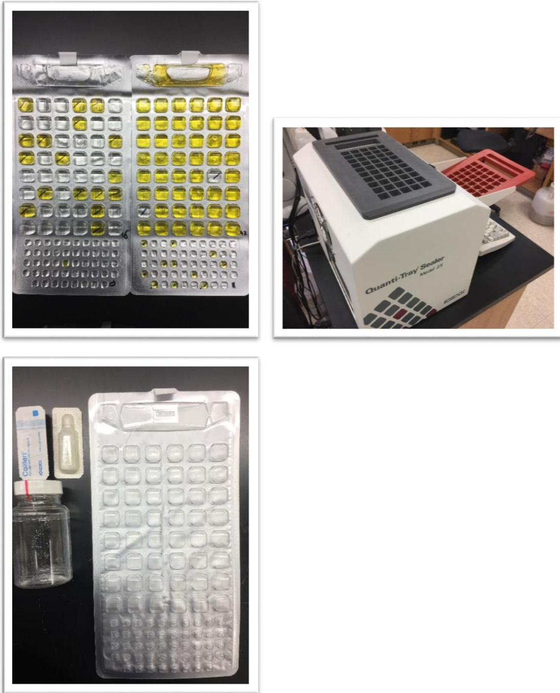
Figure 2.4: IDEXX Quanti-Tray/2000 (Quanti tray sealer, tray, vessel, and reagent).
