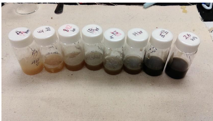
Figure A1- 19. Polycondensate Star-Ita.Gly resin. Samples taken during the time-course of polycondensation reaction.
