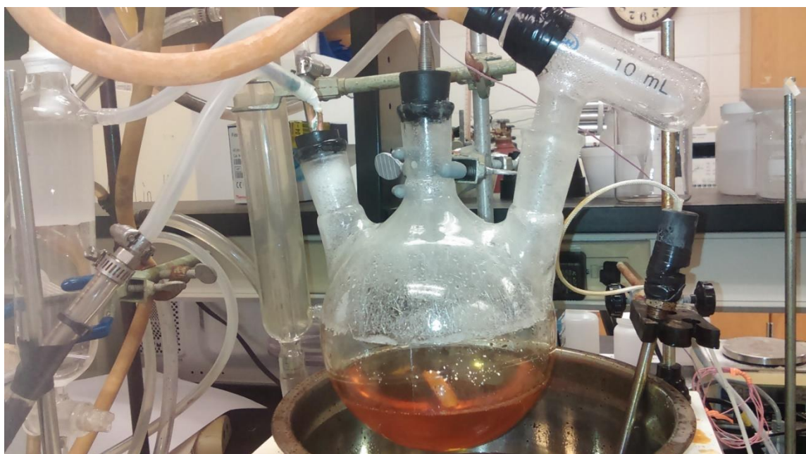
Figure A1- 4 Polycondensation's reactor with the condensed resin
