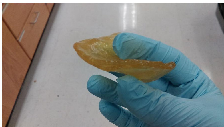
Figure A1- 14. Polycondensated Star-Ita.Gly resin with high viscosity, unsuitable for processing. More explanation in chapter 8.
