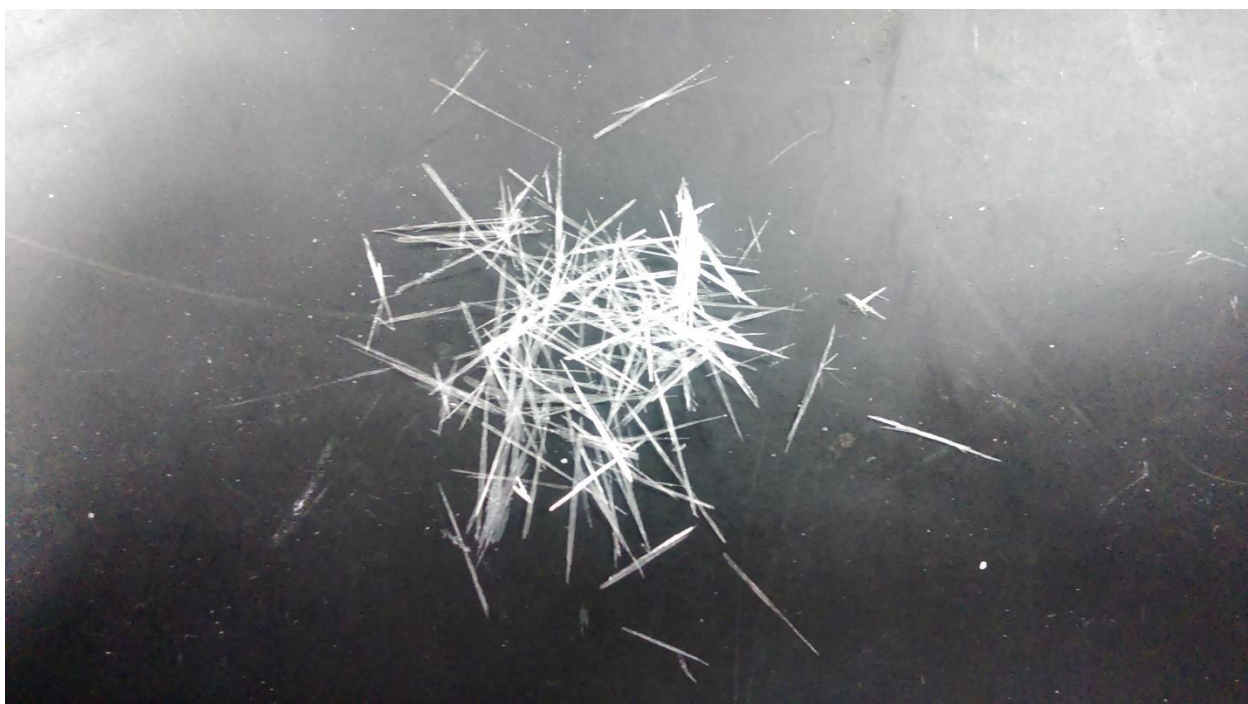
Figure A1- 16. Preparation of itaconic acid crystals inside the reactor, during the production of Star-Ita.Gly resin
