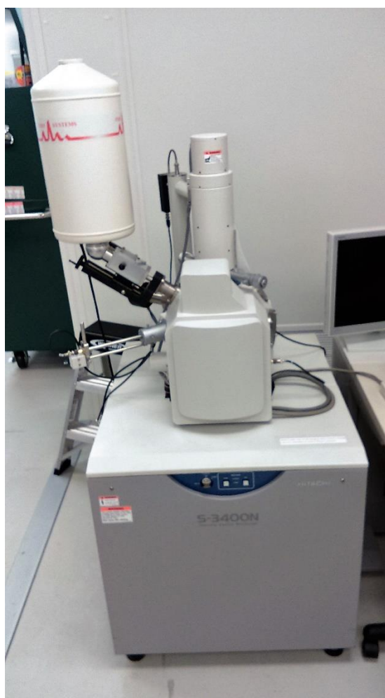
Figure A1- 7. top: sputter gold machine, bottom: SEM machine used in microscopy of the composites.
