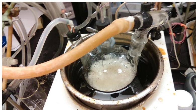
Figure A1- 13. Polycondensation's reactor with the condensed resin, for Itaconic acid based resin
