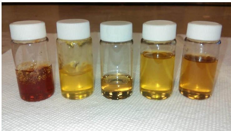
Figure A1- 20. From left to right: Star-Ita.Gly resin-Base resin, Ethanol-treated Star-Ita.Gly resin, Methanol-treated Star-Ita.Gly resin, and Allyl alcohol treated Star-Ita.Gly resin.
