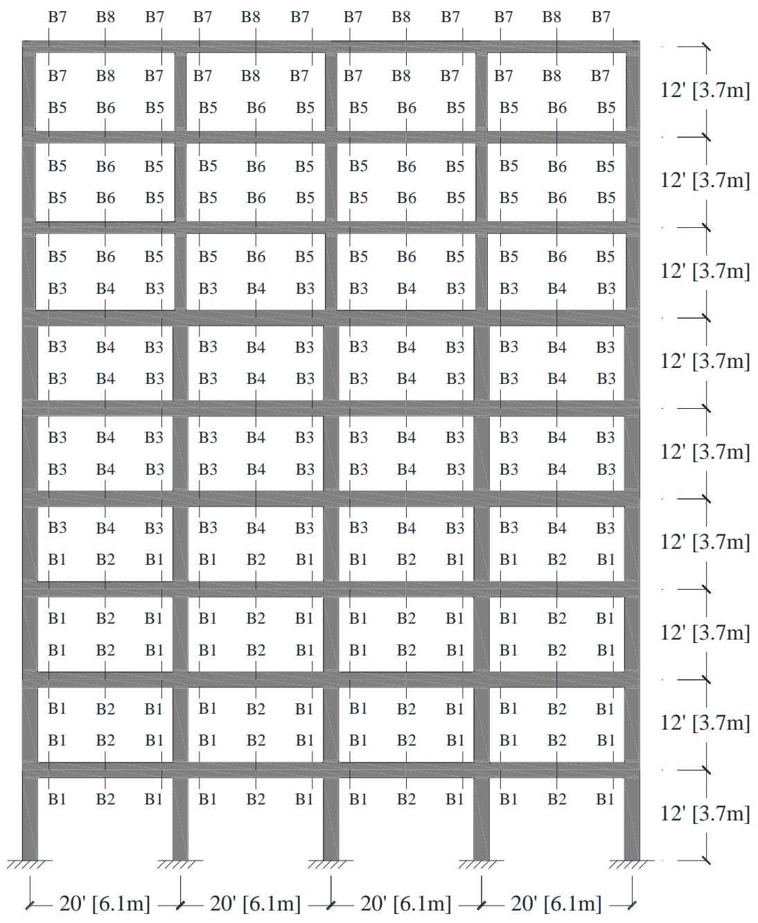
Figure 4.15- Nine-Story Ordinary Moment-Resisting Frame
