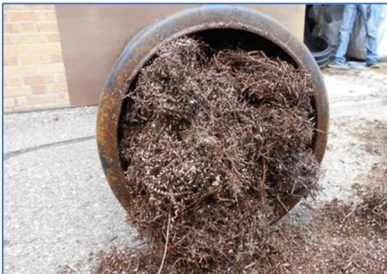
Figure 4.2 Steel shavings used as P adsorption media installed near Baltic, South Dakota
