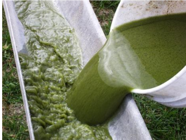
Figure 13. Microalgae harvesting using filtration technique.
