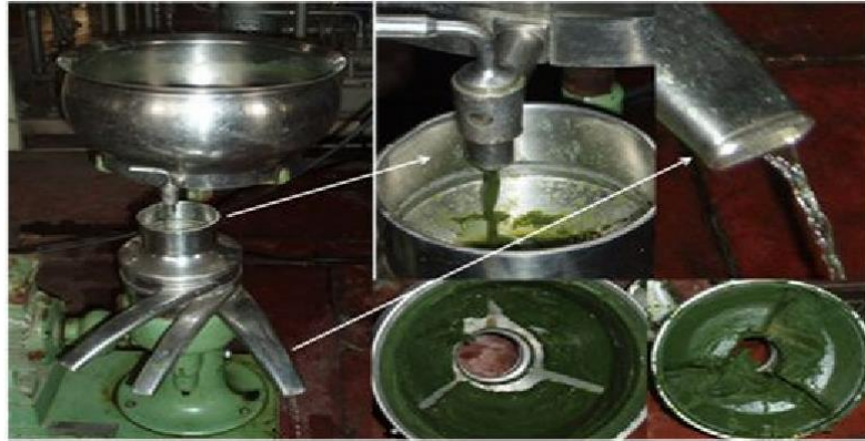
Figure 15. Harvesting micro algae through centrifugation process. (Dayan et al., 2010)
