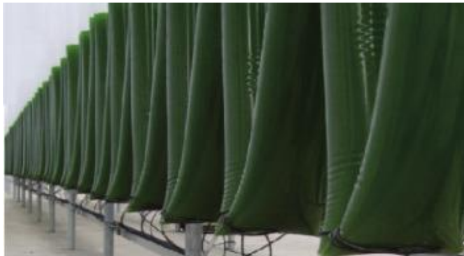
Figure 8. Plastic bag photobioreactor (Huang et al., 2017)
