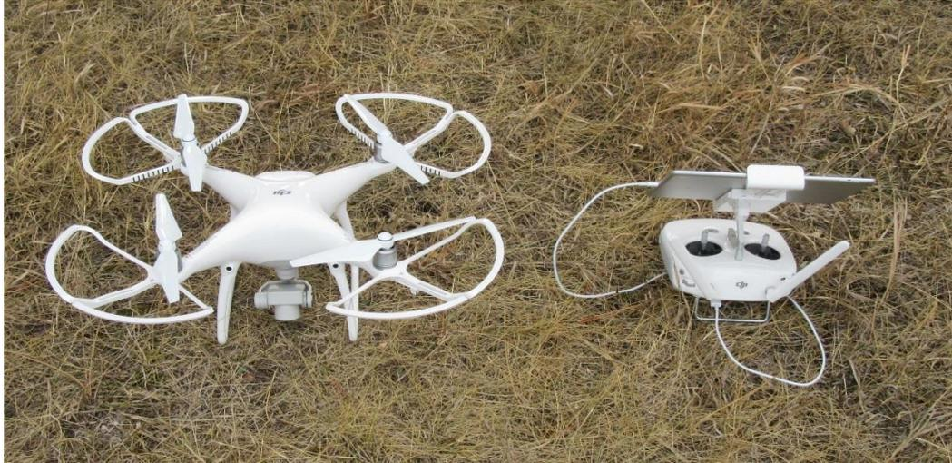
**Fig. 2-1.** Image of the DJI Phantom 4 (taken by Junwon Seo).
