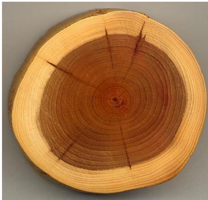
Fig 1: Yew wood ( Taxus baccata ) showing 27 annual growth rings, pale sapwood and dark heartwood, and pith (centre dark spot). The dark radial lines are small knots.
