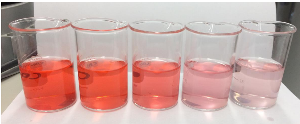
Fig. 7: Effect of pH on anthocyanins. From left to right: pH 1.0, 2.0, 3.0, 4.0, and 5.0. Color fades as pH becomes less acidic.
