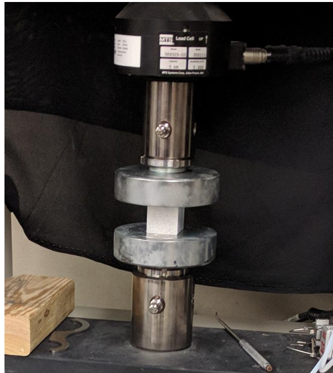
Figure 30. Compression test on 3D printed Onyx Samples
