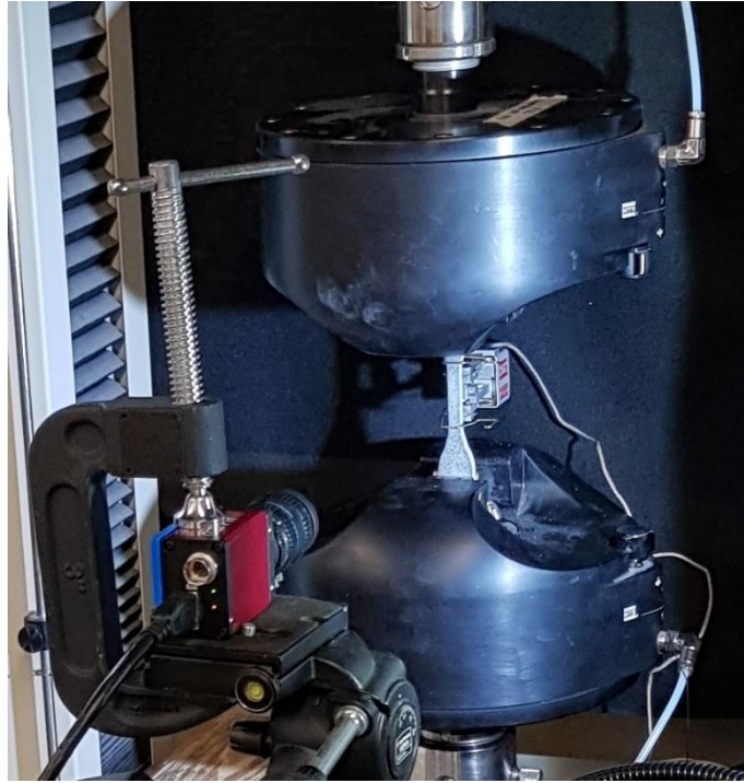
Figure 29. Tension test on 3D printed Onyx Samples
