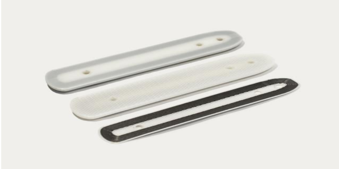
Figure 19. Printing pattern of MARK TWO printer ( Image courtesy of Mark forged )
