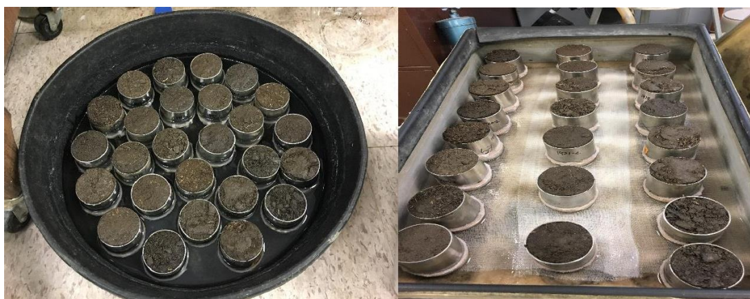
Fig. A3. Soil core samples (left) preparation for the analysis of soil water retention (right).
