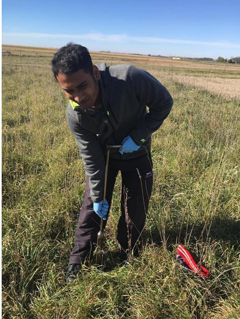
Fig. A7. Soil sample collection at various depths using hand auger at Brookings site.
