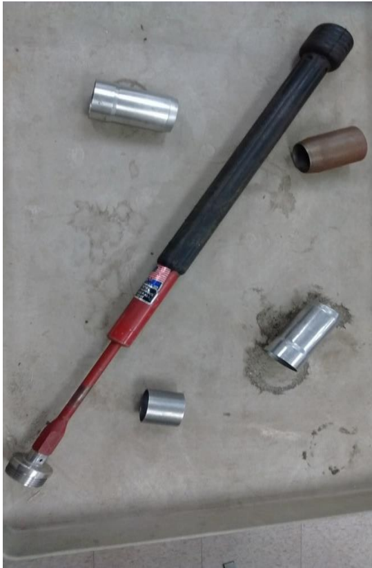
Fig. A12. Soil core sampler (left) and collection of soil core samples (right).
