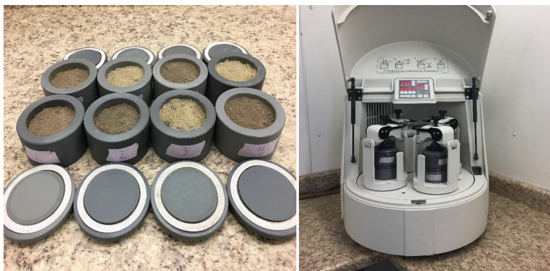
Fig. A4. Grinding of soil samples for the analysis of soil organic carbon and total nitrogen
