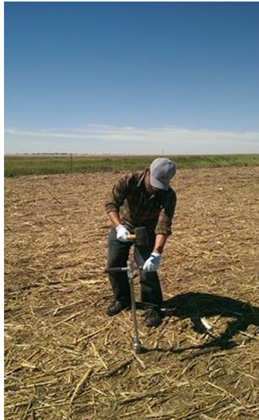
Fig. A12. Soil core sampler (left) and collection of soil core samples (right).
