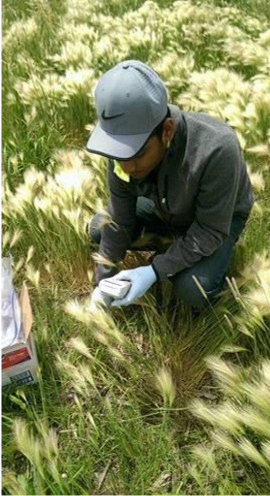
Fig. A6. Measurement of soil moisture with soil moisture meter (left) and penetration resistance using hand penetrometer (right).
