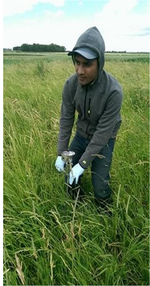
Fig. A6. Measurement of soil moisture with soil moisture meter (left) and penetration resistance using hand penetrometer (right).
