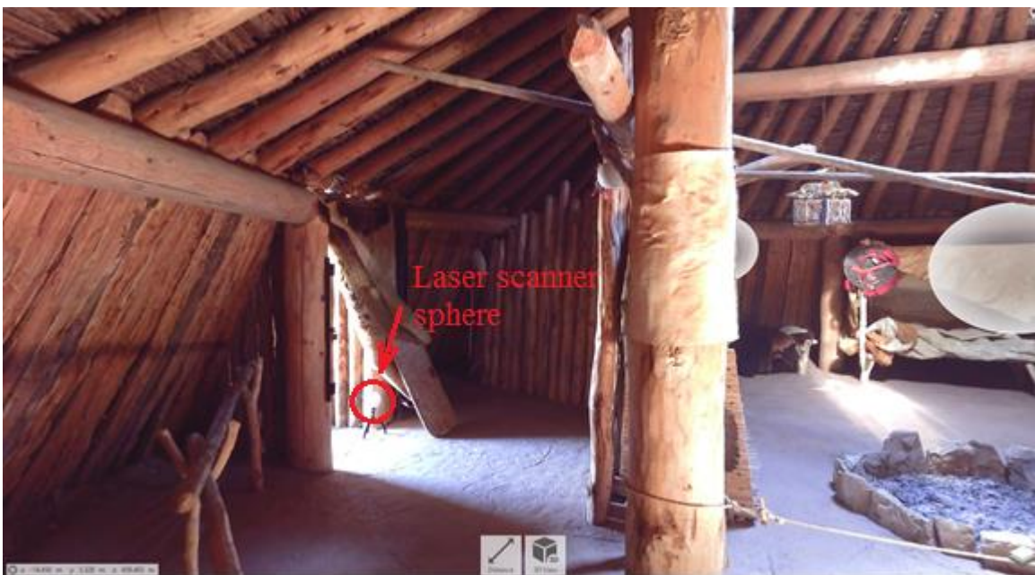
Figure C-8. Autodesk Recap rendering of entrance showing where one of the laser scanner spheres was placed (red circle).
