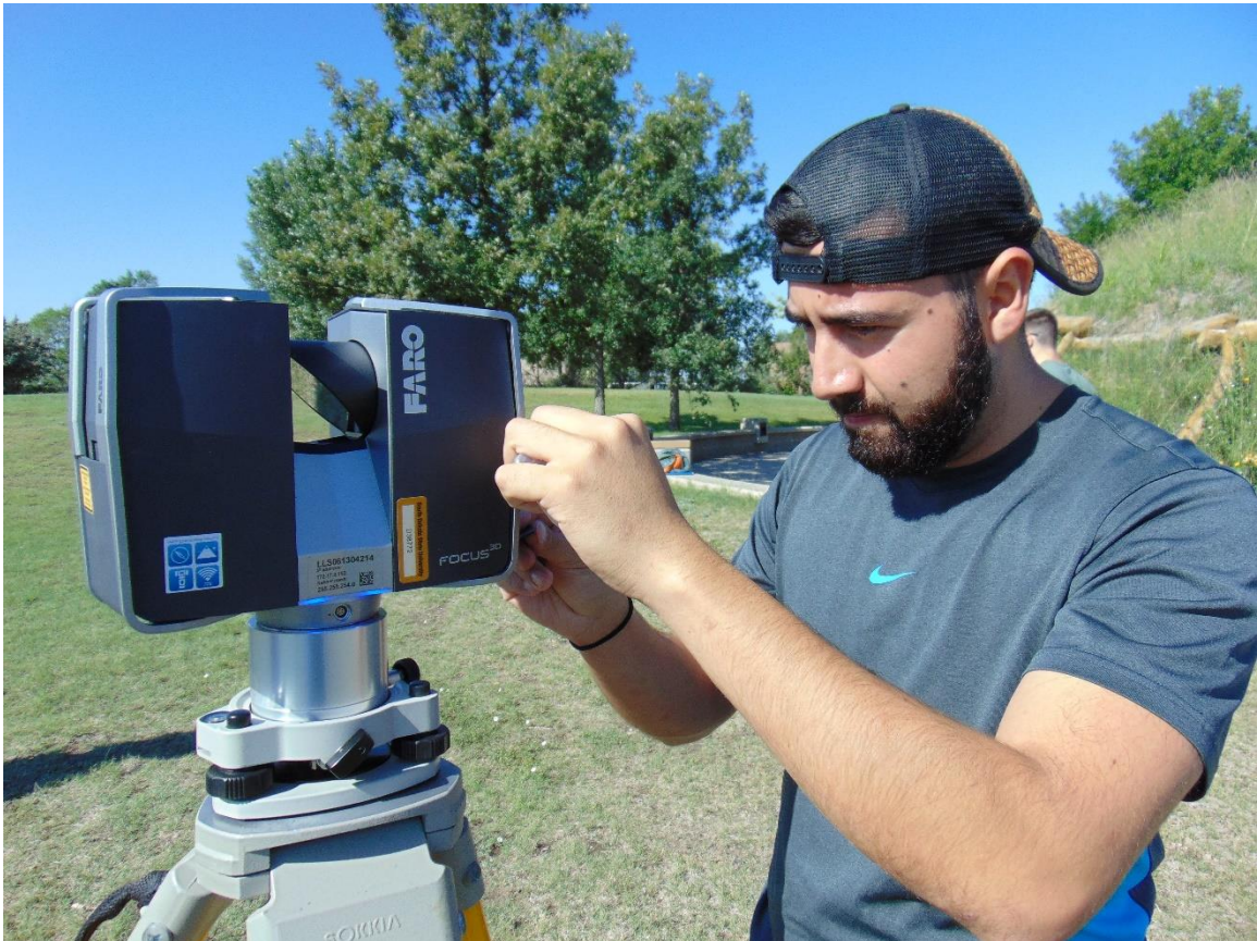
Figure C-1. Salvador Caballero, SDSU graduate engineering intern, setting FARO 3D scanner to begin scan of exterior of the reproduction earth lodge at the Knife River site, August 2017. (photo: Joanita Kant)
