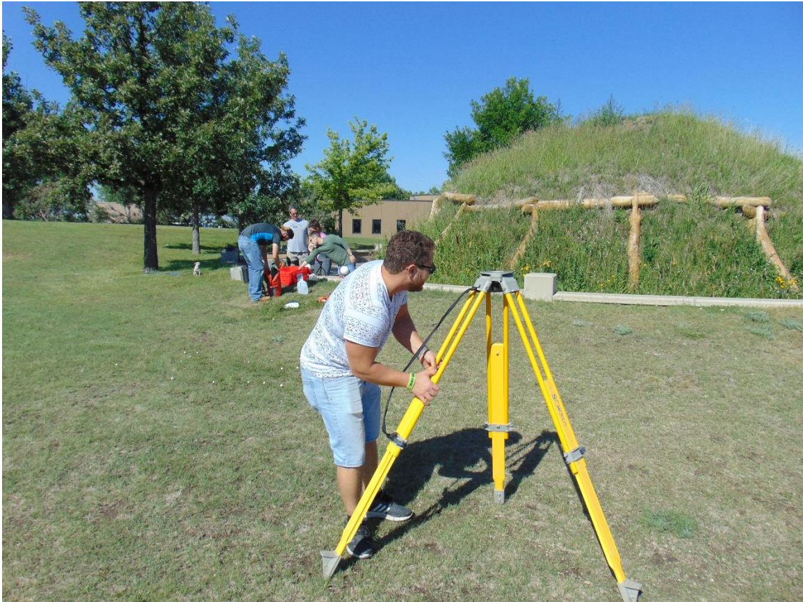
Figure A-4. (L-R) Yazen Hindieh, SDSU graduate engineering intern, setting tripod for FARO 3D apparatus to scan exterior of reproduction earth lodge at the Knife River site, August 2017. (photo: Joanita Kant)
