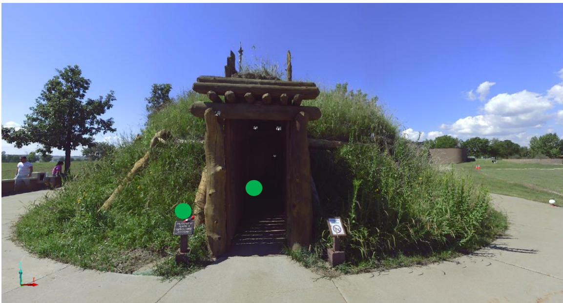
Figure C-7. Autodesk Recap rendering of entrance of reproduction earth lodge at the Knife River Village National Register. The green neon dots represent the laser scanner reference spheres.
