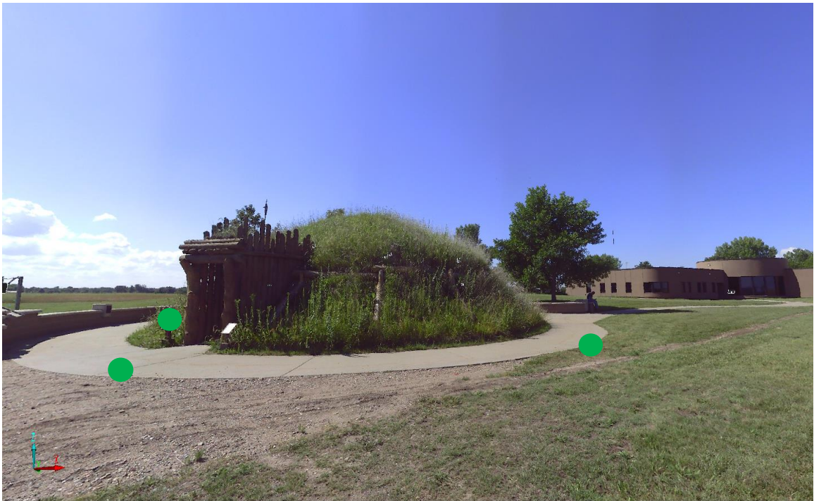
Figure C-6. Autodesk Recap rendering of reproduction earth lodge at the Knife River site. The small green dots are the laser scanner reference spheres positioned to scan this section of earth lodge.
