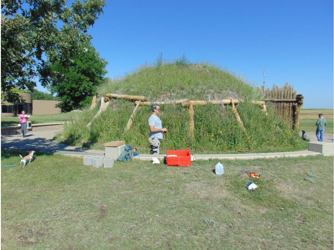
Figure A-6. (L-R) Keely Moriarty, SDSU undergraduate engineering student; Freddy Moran, SDSU graduate engineering intern, and Calvin Wampol, SDSU graduate engineering intern, placing the laser scanner reference sphere set around exterior of reproduction earth lodge at the Knife River site, August 2017. (photo: Joanita Kant)
