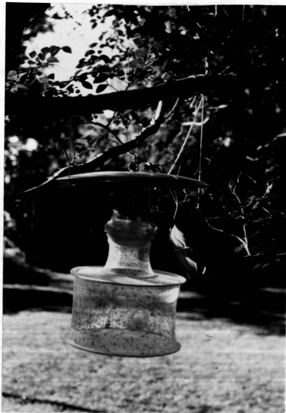
Figure 3. New Jersey Mosquito Light Trap with a dry ice block hanging beside the trap
