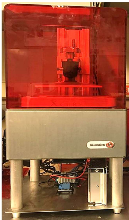
Figure 17. Modified X-Cube LCD 3D Printer
