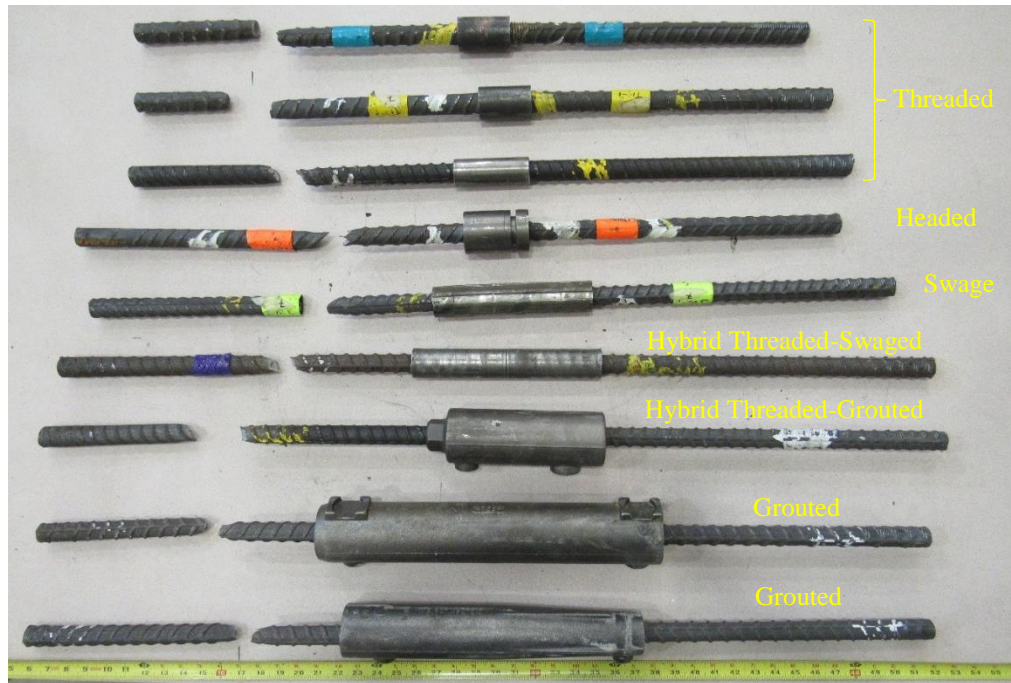
Figure 2-1. Different mechanical bar splice products
