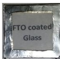
Figure 2.6. FTO-glass substrate bordered with Al foil to use inside MW reactor
