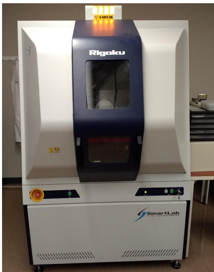
Figure 2.9. Rigaku Smartlab X-ray diffractometer
