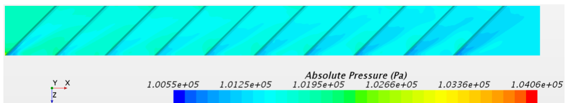
Figure 4.28. Absolute Pressure contour plot for 45° pentagon rib
