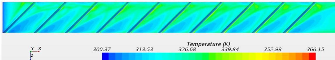
Figure 4.61. Temperature contour plot for 45° pie-slice rib pointing upstream
