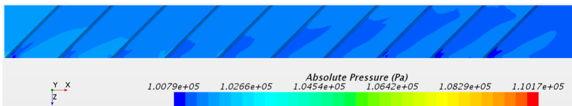
Figure 4.60. Absolute Pressure contour plot for 45° pie-slice rib pointing upstream
