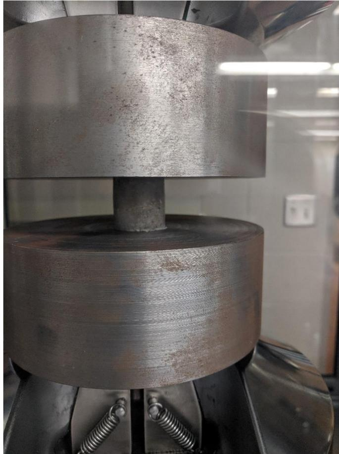
**Figure 16. Compression Sample in Test Fixture**
