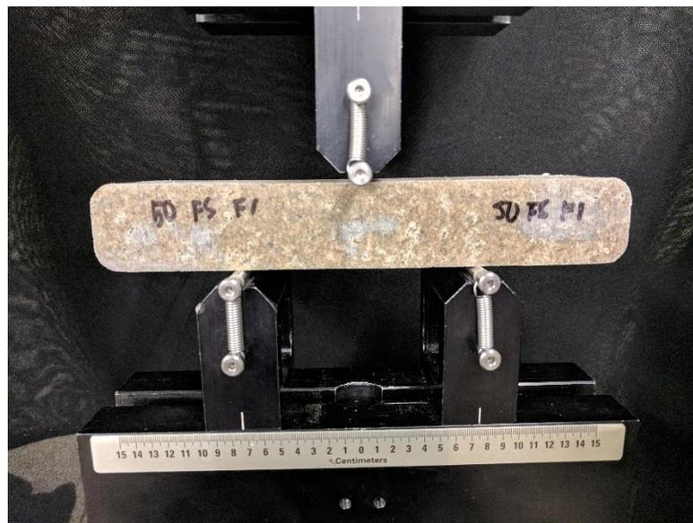
**Figure 15. Flexural Test Setup**
