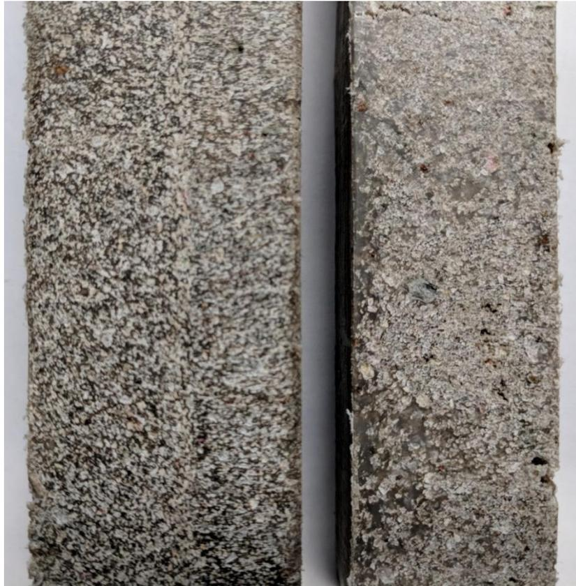
**Figure 50. Comparison of Printed (left) and Molded (right) Flex Samples of 30% HDPE/FS**
