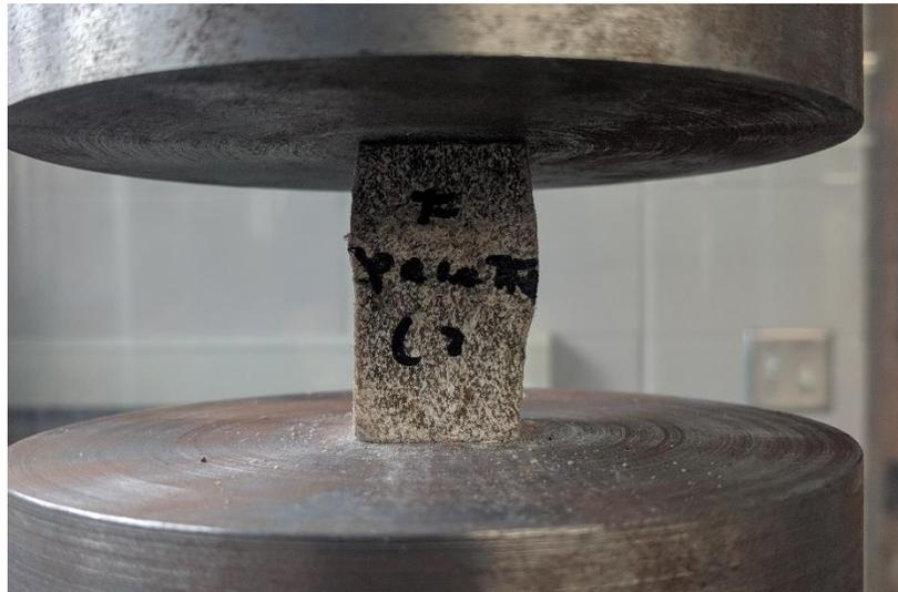
**Figure 53. Printed Compression Sample After Failure**
