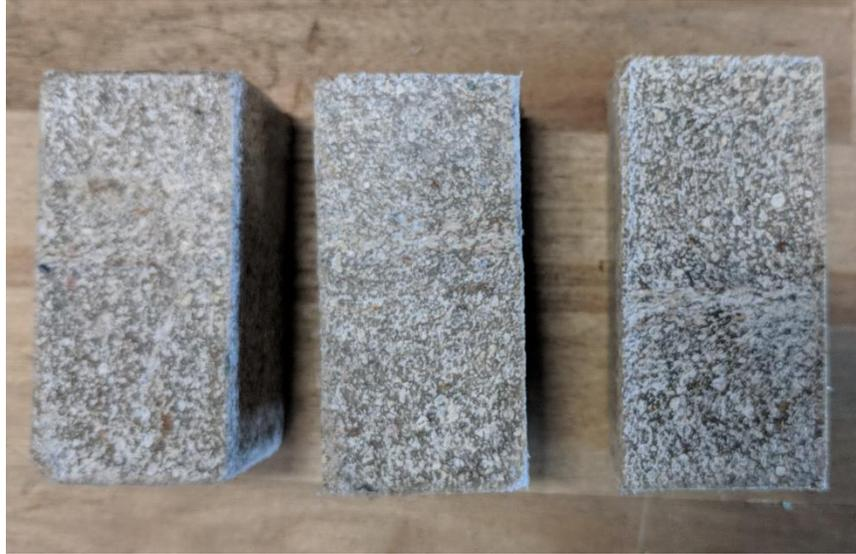
**Figure 52. Printed Compression Samples**
