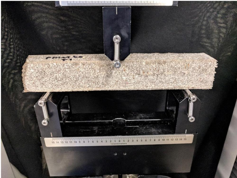
**Figure 51. Printed Flexural Sample in Test Fixture**
