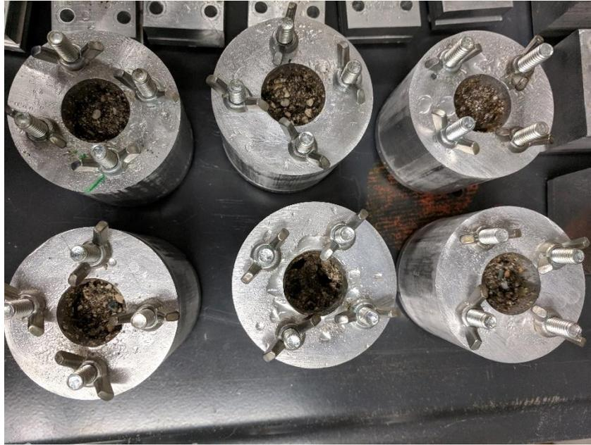
**Figure 14. Melted Compression Samples in Molds**
