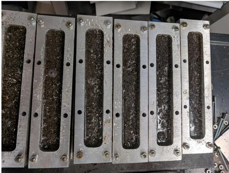
**Figure 13. Melted Flex Samples in Molds**
