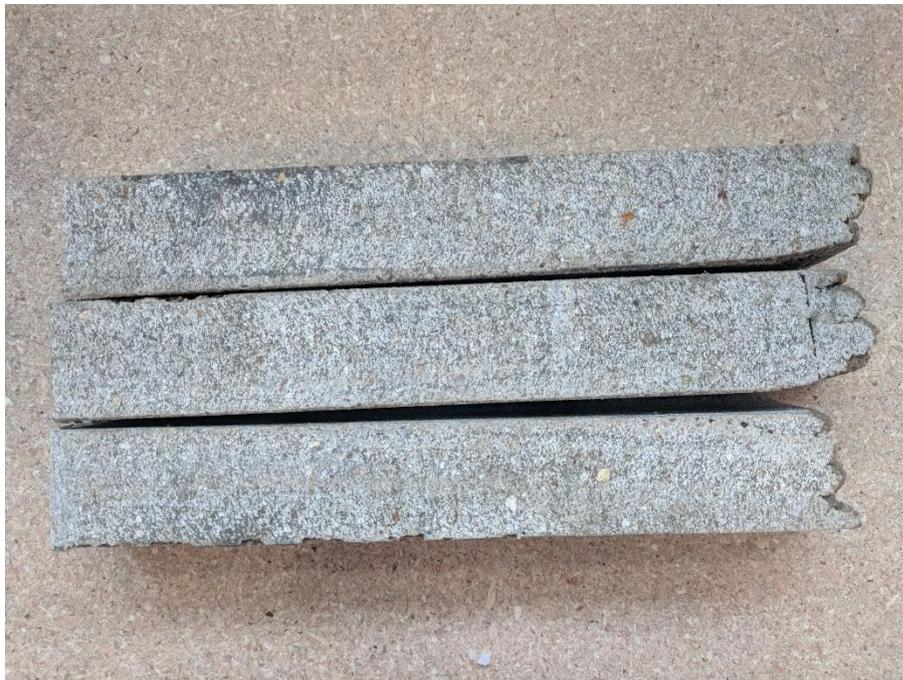
**Figure 19. Flex Samples Cut from Printed Block**
