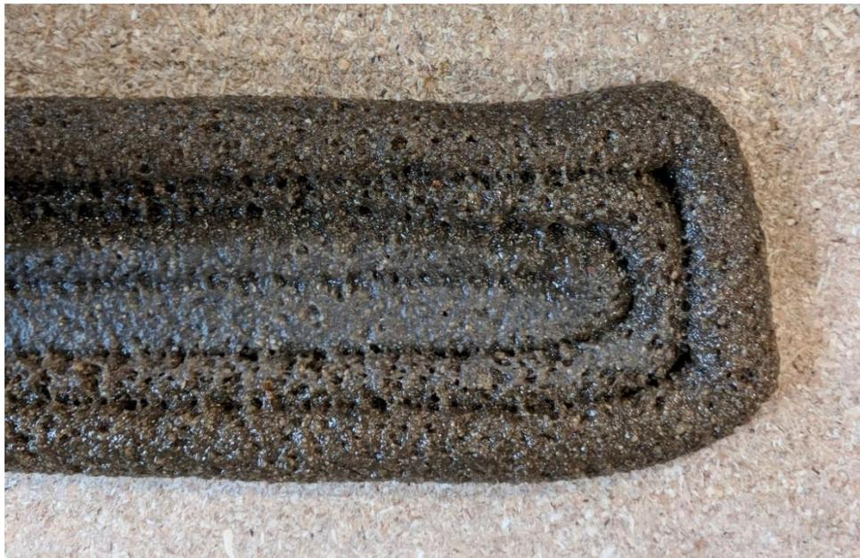
**Figure 47. Second Test Print Line Overlap**
