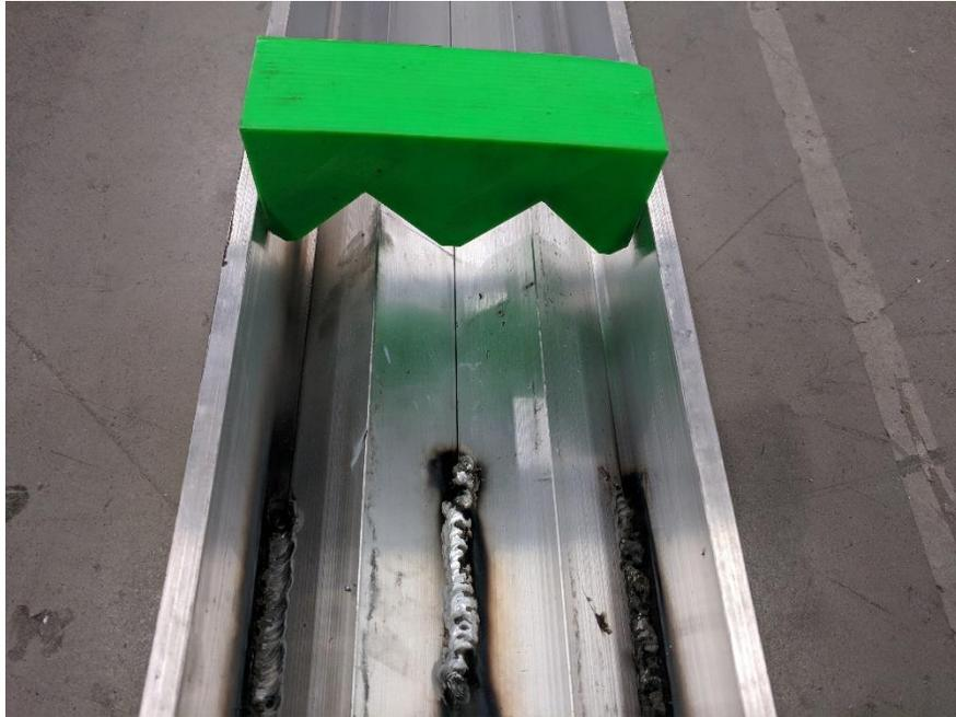
**Figure 34. X-Axis Rail Jig Assembly**
