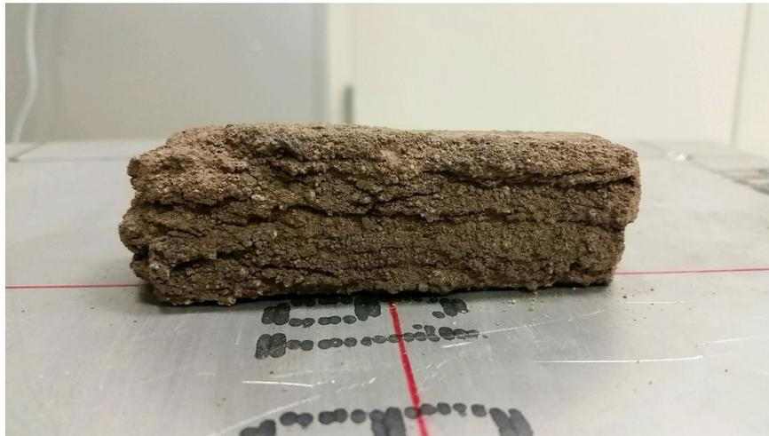
**Figure 4. Printed Sulfur Sample**
