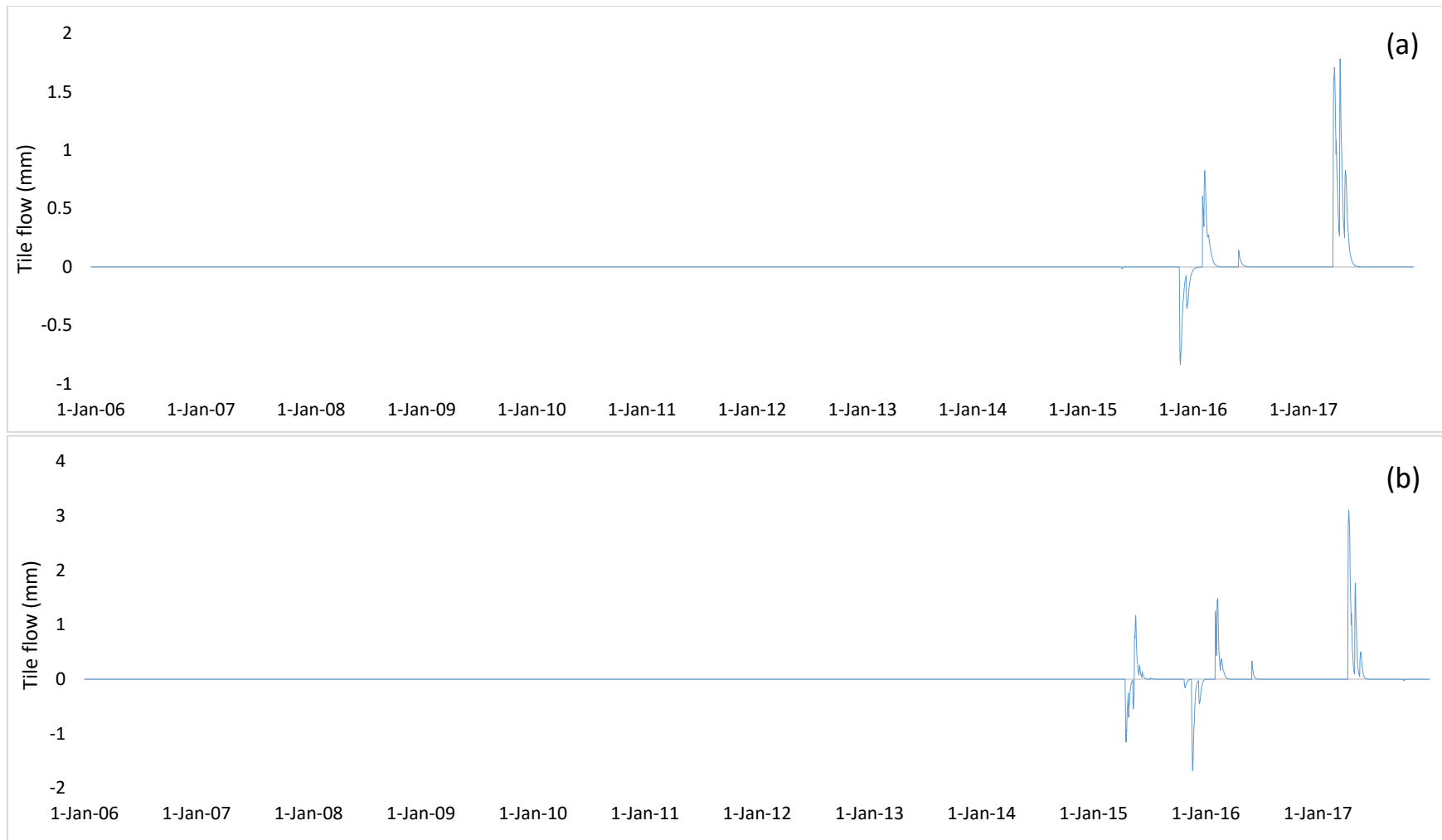
Figure 3.13 Difference in daily tile flow for MG2 and MG1 management schedules throughout the study period for the eastern (a) and western half (b). Positive values represents greater flow in MG2 than MG1 and vice versa.
