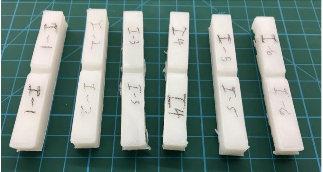
Figure 4.9. Impact test specimens
