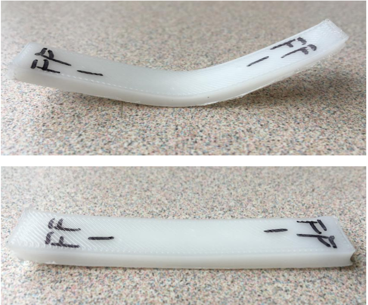
Figure 5.7. HDPE flexural specimen immediately after the test (top image) and several minutes after the flexure test (bottom image).
