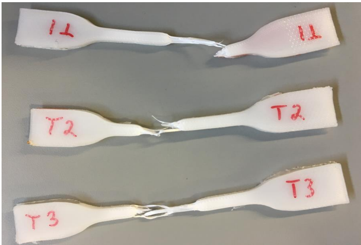
Figure 5.2. Fibrous strands after tensile failure
