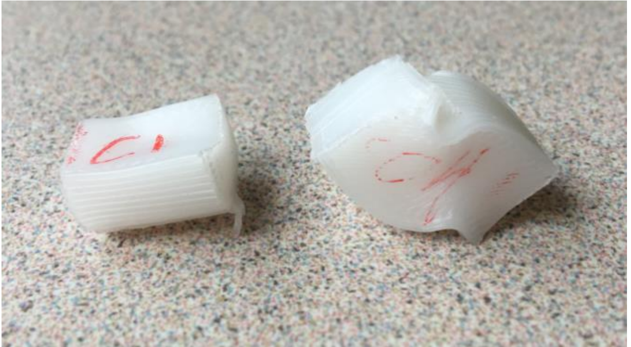
Figure 5.4. Compressive HDPE specimens after load testing (loaded perpendicular to the layers on the left and loaded parallel to the layers on the right)
