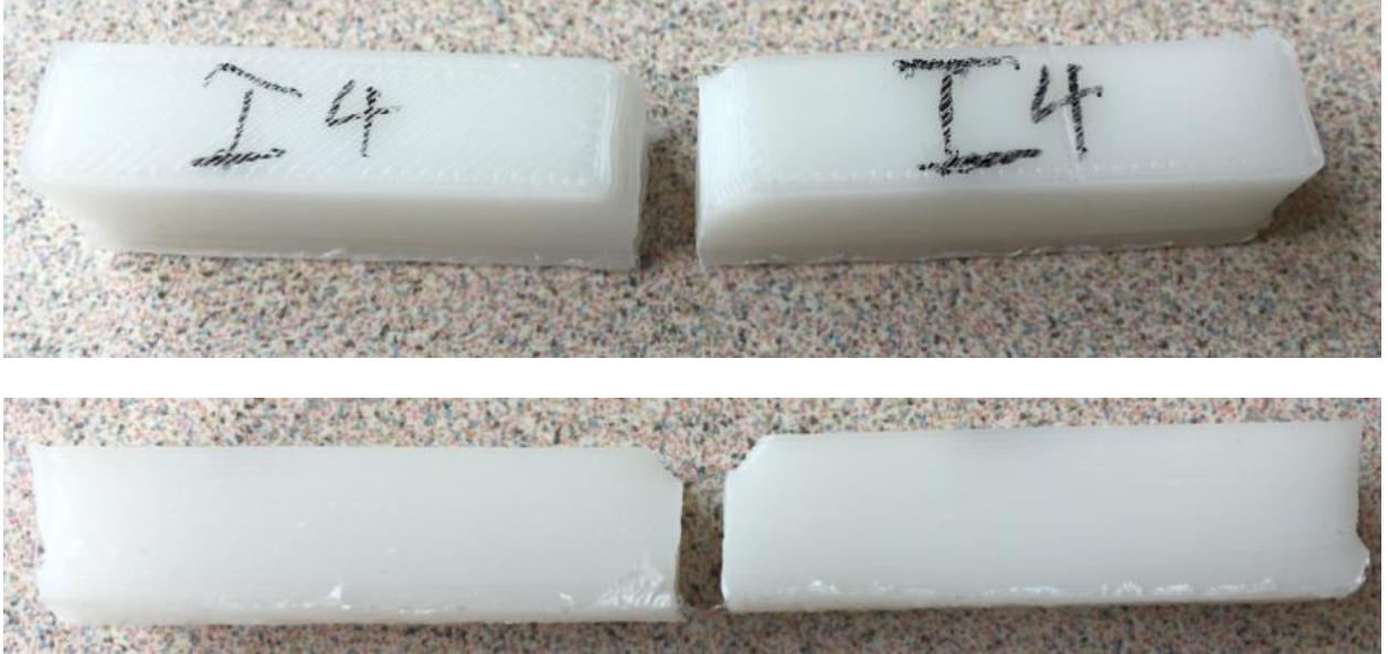
Figure 5.5. HDPE impact specimen after test.
