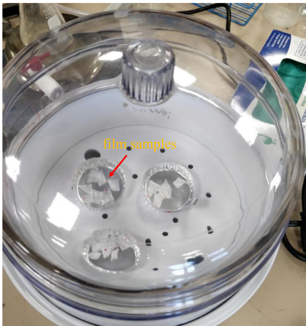
Figure 2.5 Samples of pure PLA films and PLA/3% CNC films inside the desiccator at 95% RH and room temperature.
