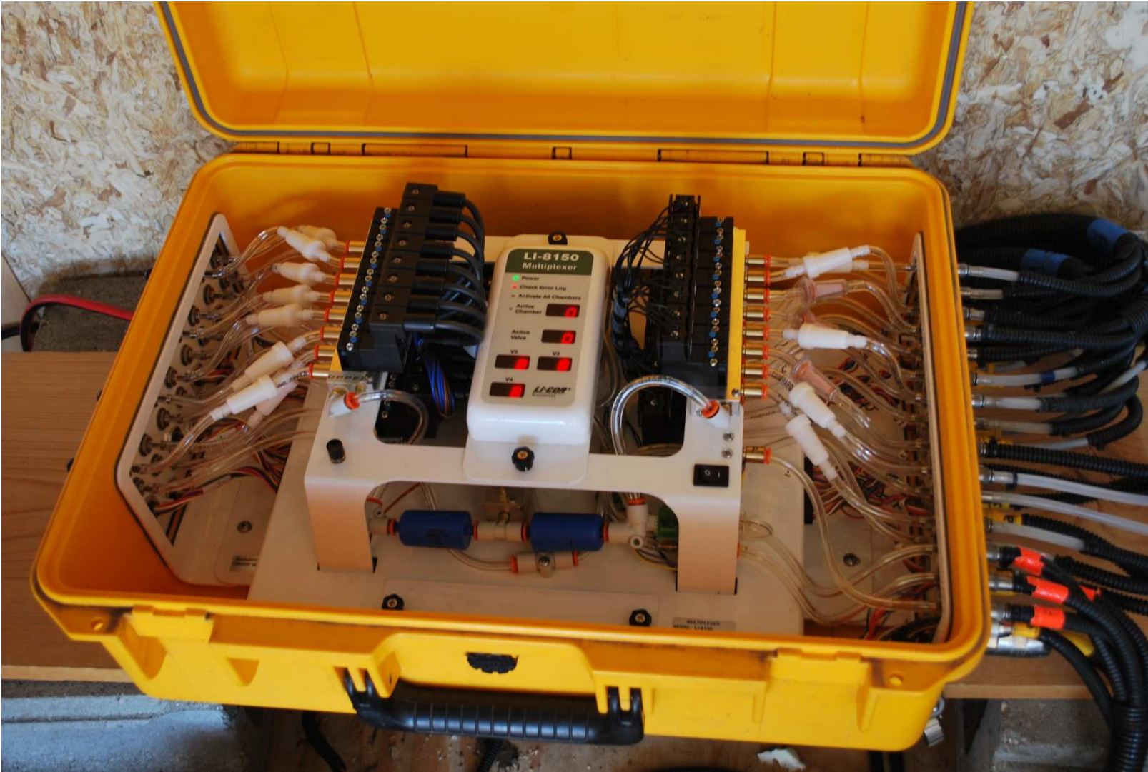
Supplemental Picture 3: The LI-COR LI-8150 16 port multiplexer. This multiplexer switched gas samples automatically.
