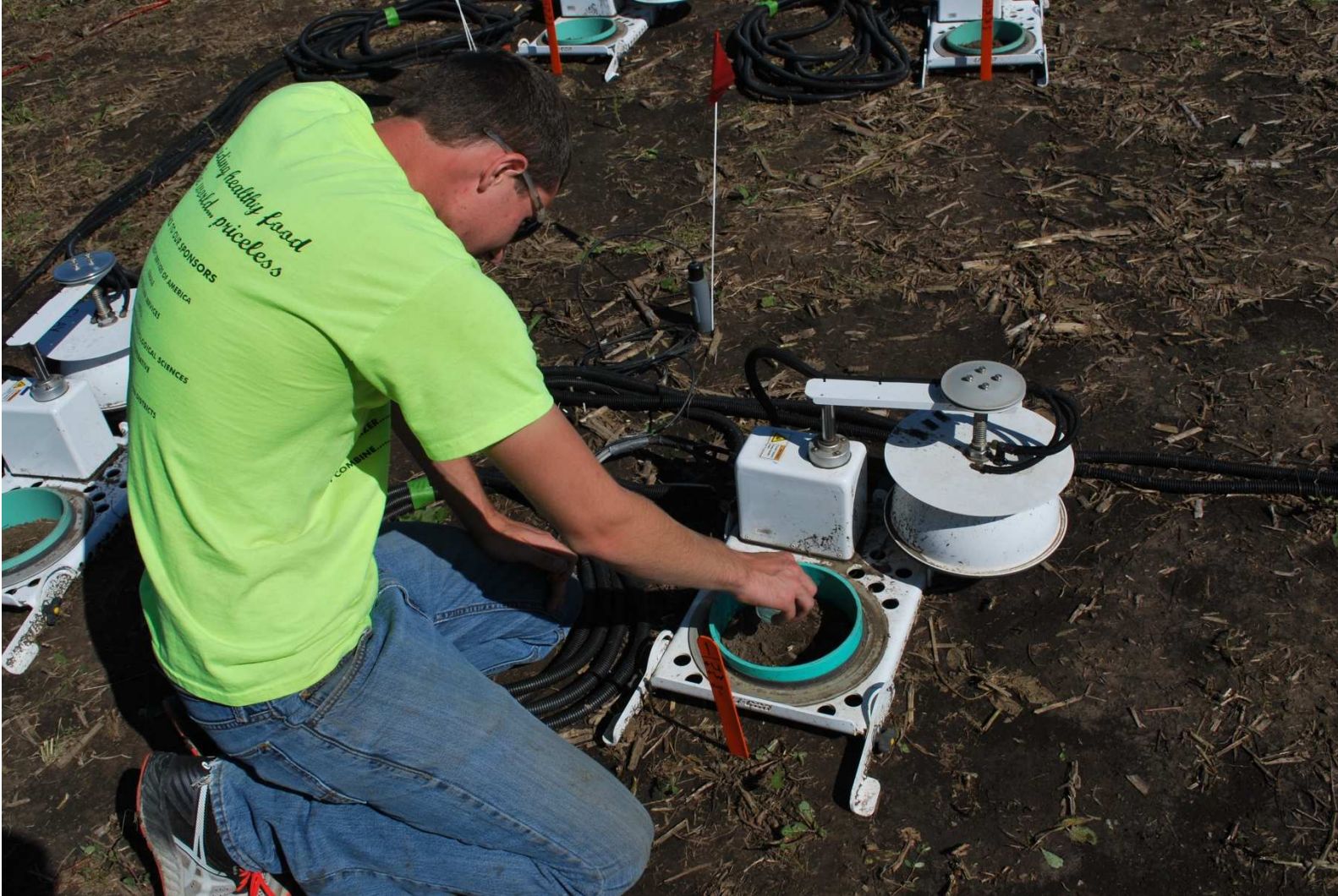
Supplemental Picture 5: This picture shows the application of the urea fertilizer in the field to the LI-COR LI-8100-104 long term chambers. The urea fertilizer was dissolved in water before application.
