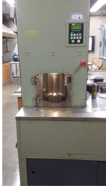
Figure 3.6 Compaction of sample using Superpave ® gyratory compactor
