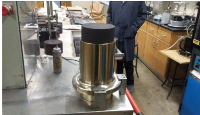
Figure 3.6 Compaction of sample using Superpave ® gyratory compactor
