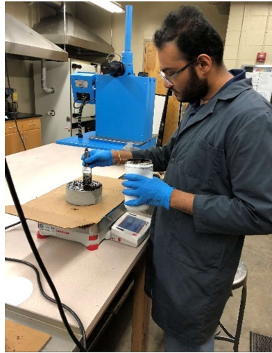
Figure 3.13 Applying tack coat on bottom layer sample
