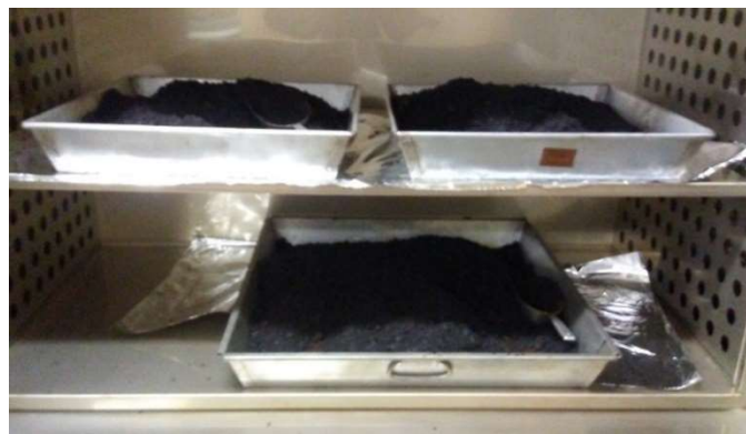
Figure 3.3 Heating the asphalt mix inside an oven at 165° C
