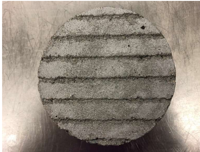
Figure 3.12 Grooved PCC bottom layer sample
