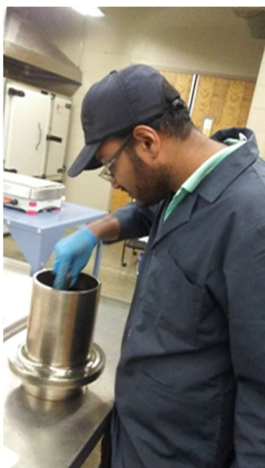
Figure 3.4 Weighing the asphalt mix inside the mold
