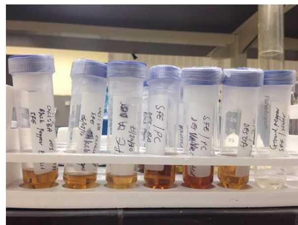
Figure 3.23. Liquid-liquid extract of piperine in ethyl acetate.
