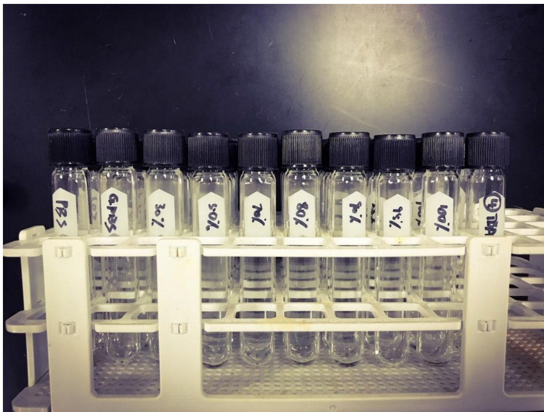
Figure 5. Picture of SEM pre-treatment solvents. The solvents left to right: 0.01M PBS, 2.5% GPBS, ethanol (30%, 50%, 70%, 80%, 90%, 95%, 100%), 100% TBA.
